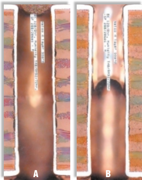
Figure 5. European (K8) Automotive Specification \leq 15\% Resin recession requirement. A: N4000-6/+ 30% recession (fail), B: N4000-7/11% recession (pass).
