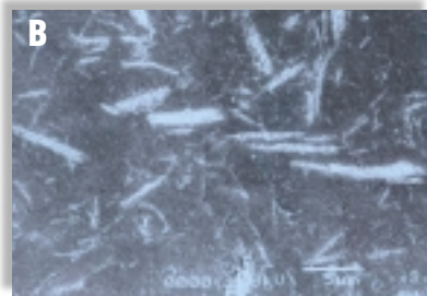
Figure 1. N4000-7 Filled Resin System. A: Appearance at 1000X B: Appearance at 3000X
